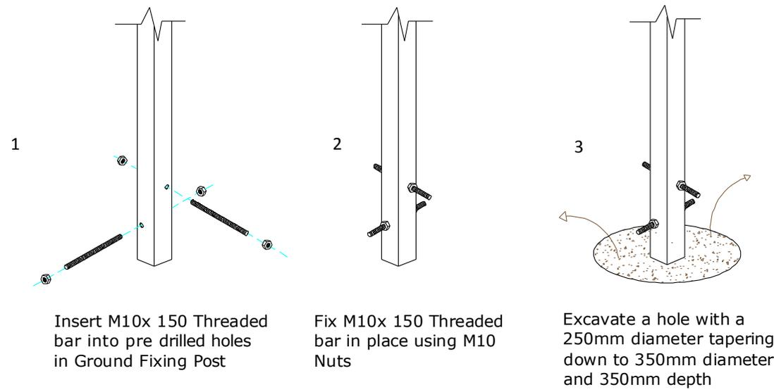
Foundations should not present a hazard. These foundations are recommended as a guide, for more information on foundation details for various surface see Part 7 of BS EN 1176.
